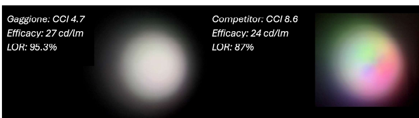
Figure 8: Comparison of color mixing optics.
